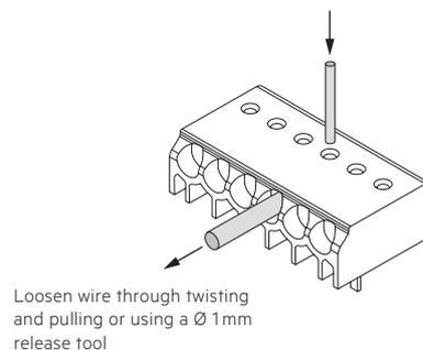
Loosen wire through twisting and pulling or using a Ø 1 mm release tool
